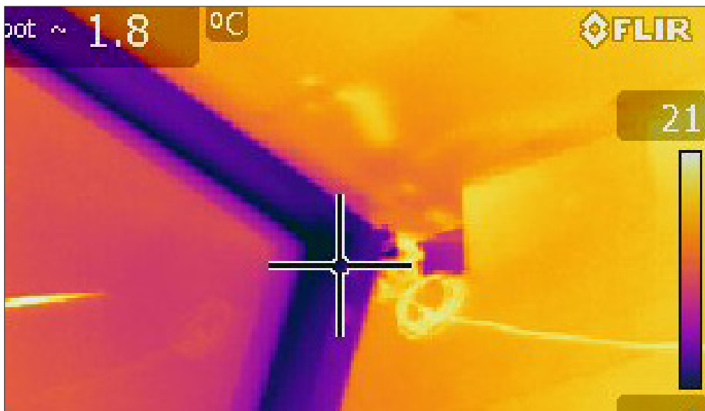
Image: Thermal Camera Image showing Heat Escaping out of the Hole
